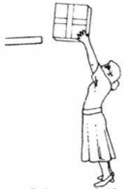
Over-reaching while handling (i.e lifting from below mid strengths thigh or above shoulder height)
