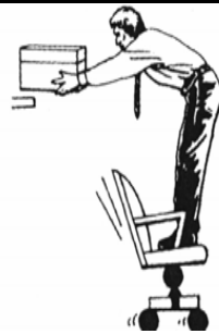
Handling on unstable work surface under foot.
