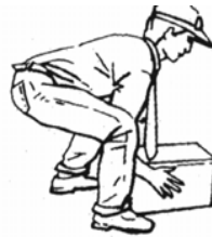
Insecure grip and poor lifting position with feet too close together while handling
